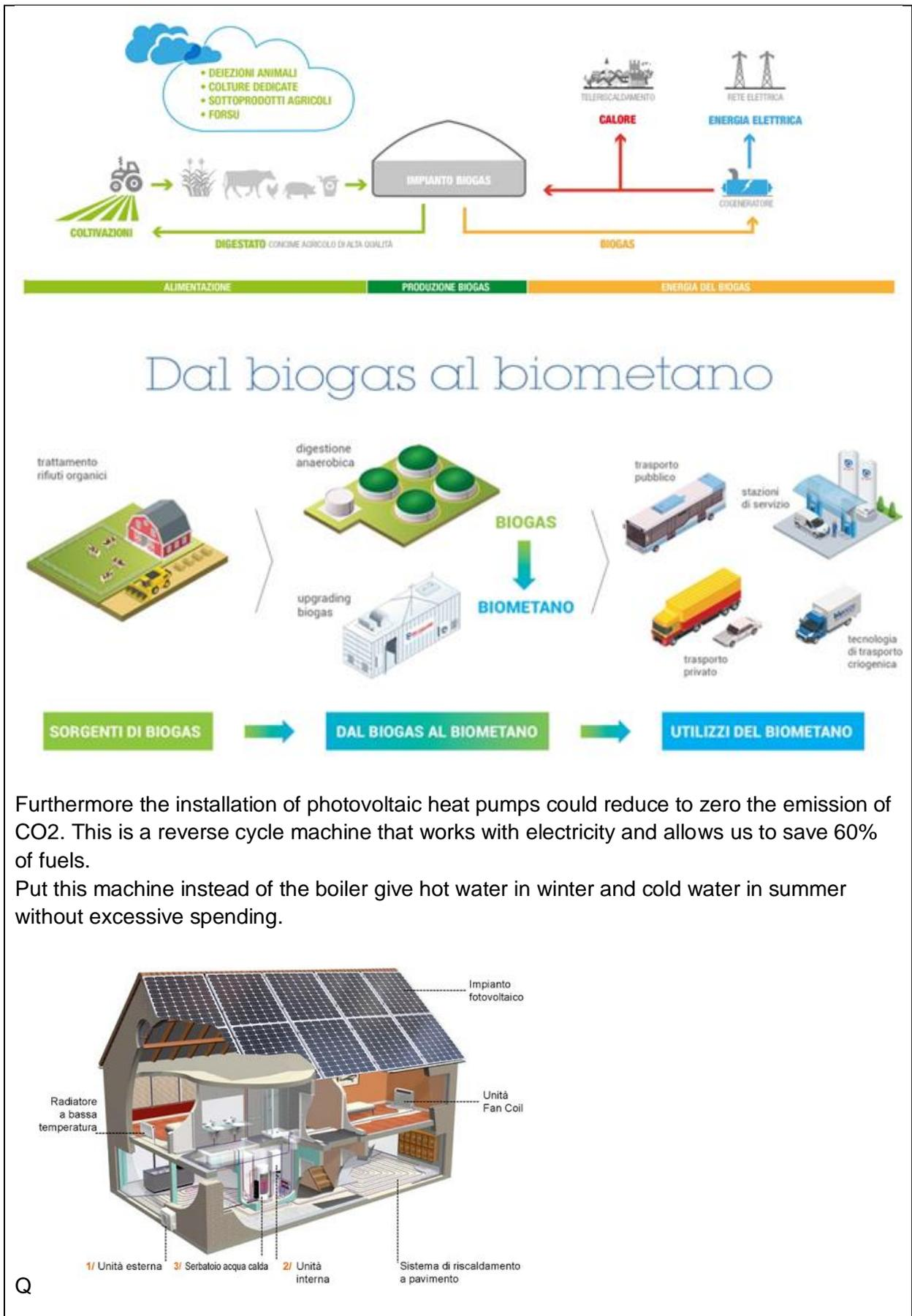
Furthermore the installation of photovoltaic heat pumps could reduce to zero the emission of CO<sub>2</sub>. This is a reverse cycle machine that works with electricity and allows us to save 60% of fuels.
